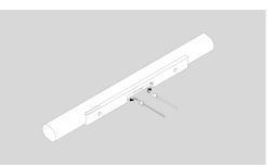
Slide the soundbar down so the knobs fit into the slots on the wall bracket. Make sure the touch controls are facing up and the soundbar is fully seated.
